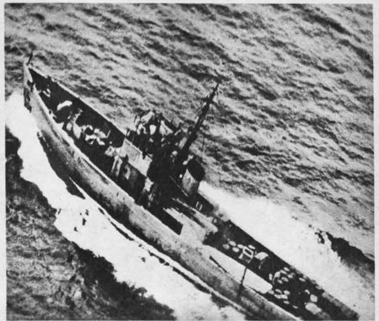
Fleeing SCS-1 carries load of depth charges, two chutes for dropping them at stern. Raked stack is set close behind ramshackle box bridge.
